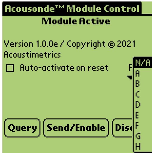
**Figure 20. The Module page showing that a module is active, with the preset menu displayed.** The list of presets is offered by the user interface, not the module itself. A given module may support only a subset of the presets listed, or it may not support presets at all.
