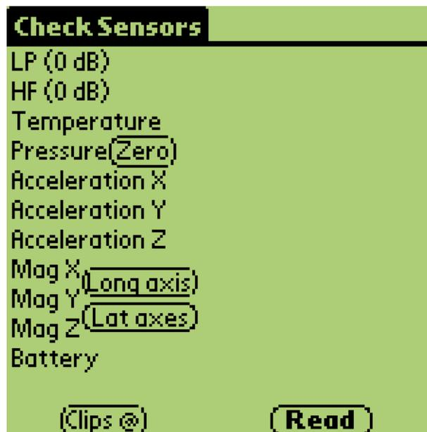
**Figure 26.** Checking current calibrated sensor readings. The **Clips@** command returns the maximum levels/reading possible for each channel.
