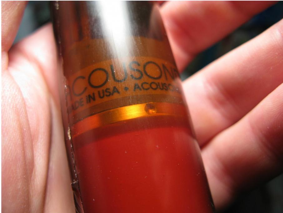
**Figure 10. Acousonde 3A battery-housing bulkhead with “up” orientation dimple.** Besides being the location of the orientation dimple, the battery-housing bulkhead is the strongest part of the Acousonde 3A and an ideal location for a securing strap.
