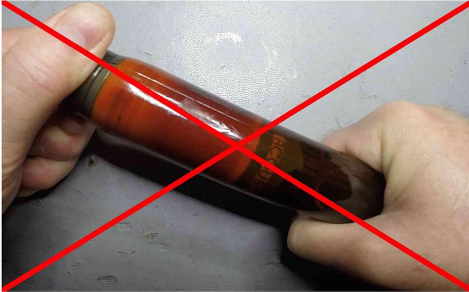
**Figure 6. Incorrect technique for tightening battery cap on Acousonde 3A.** Grasping the Model 3A far from the battery cap while tightening the cap applies a mechanical twist to the embedded electronics. Excessive twist may result in permanent damage.
