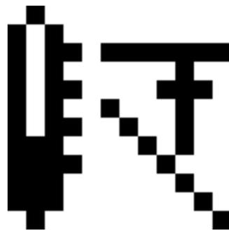
**Figure 27.** Icon indicating thermal-drift pressure compensation is active. The icon will display in the **Pressure** row of the **CHECK SENSORS** page after current sensors readings have been retrieved from the Acousonde.
