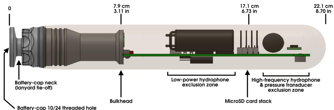
**Figure 11. Location of securing/tie-off points on Acousonde 3A.** The bulkhead region can tolerate much more mechanical stress than the MicroSD card stack region. Avoid securing anything in the exclusion zones. The “flange” type battery cap is shown.
