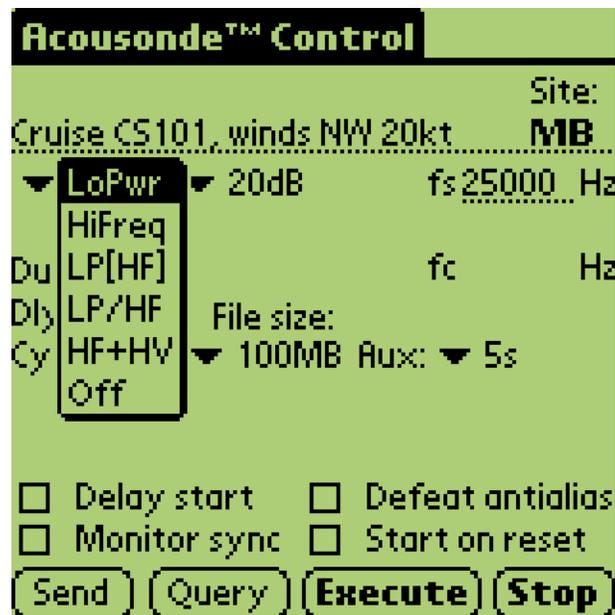
**Figure 8. Acoustic sampling programs available via the PalmOS interface.** The user has requested an acoustic sampling rate of 25000 Hz with a gain of 20 dB, and has filled in the **Site** and **Deployment Title** fields. The auxiliary sampling rate is set for a 5-second period, but other choices are available as shown in Figure 9.
