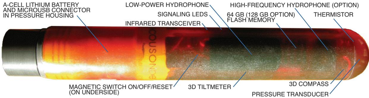
Figure 1. Acousonde 3A.
