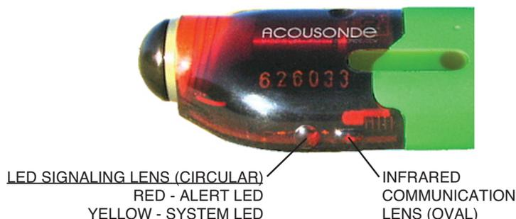
**Figure 3. Location of signaling and infrared communication lenses.** An Acousonde 3B is shown; the lenses are similar on an Acousonde 3A.
