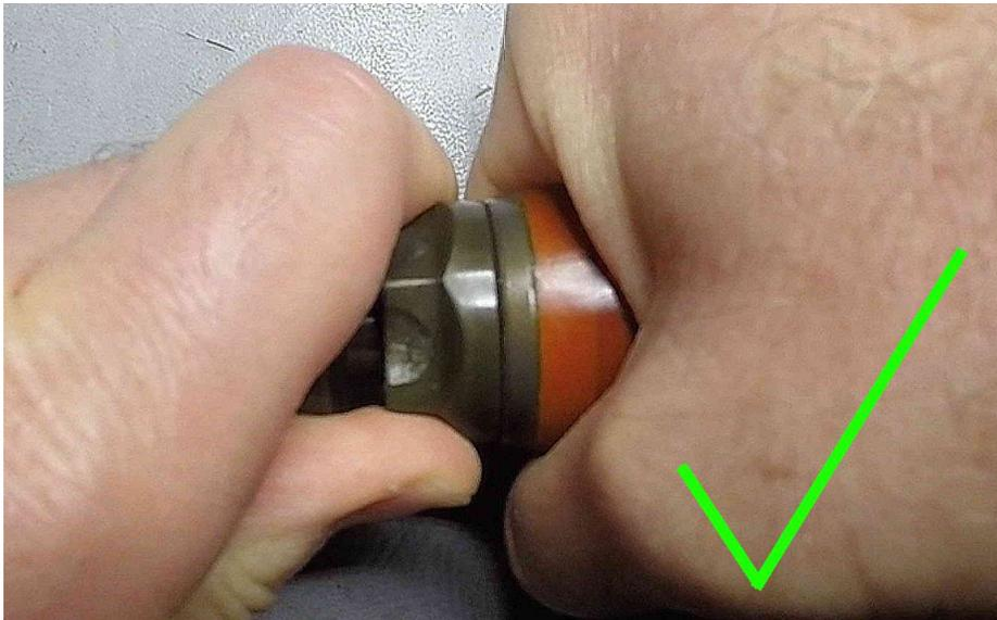
**Figure 7. Correct battery-cap tightening technique for Acousonde 3A.** Grasping the Model 3A near the battery cap minimizes twist to the embedded electronics.
